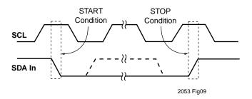
Figure 9. I<sup>2</sup>C Start and Stop Timing
