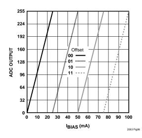
Figure 6. Quarter Scale (code 01<sub>BIN</sub>) with Offset
