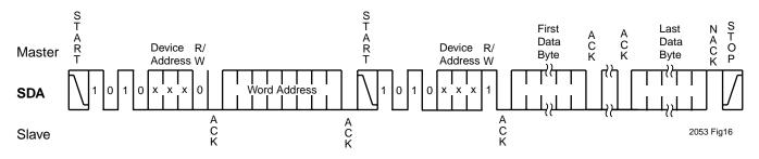
Figure 16. Look-up Table Sequential Read with Dummy Write
