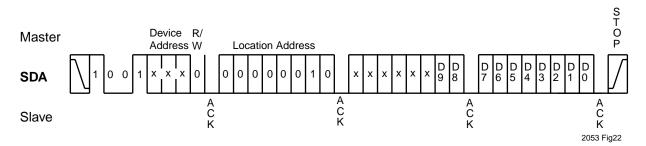
Figure 22. 10-Bit DAC Nonvolatile Register Write
