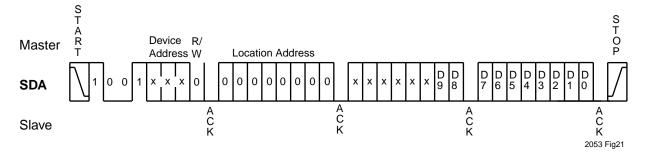
Figure 21. 10-Bit DAC Volatile Register Write
